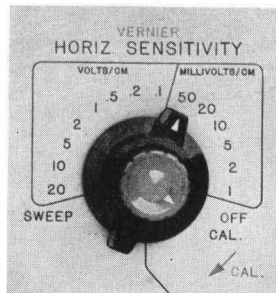
Fig. 8. Sensitivity of vertical and horizontal amplifiers is controlled by single, direct-reading switches. Sensitivity verniers are concentric with switch knob.
